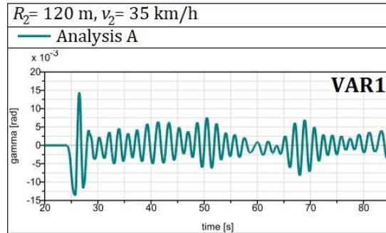
Fig. 4. Results of the Analysis\_A for the VAR1 bogie, Rc\_II
