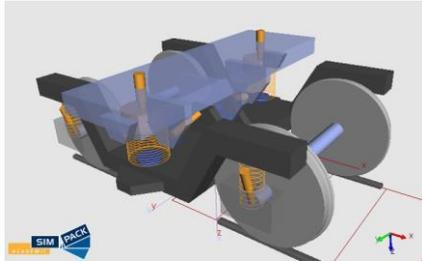
Fig. 1. MBS model of the bogie
