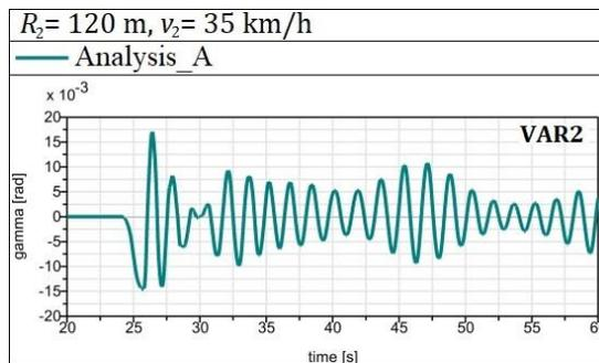
Fig. 6. Results of the Analysis\_A for the VAR2 bogie, Rc\_II
