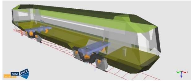
Fig. 2. MBS model of the locomotive
